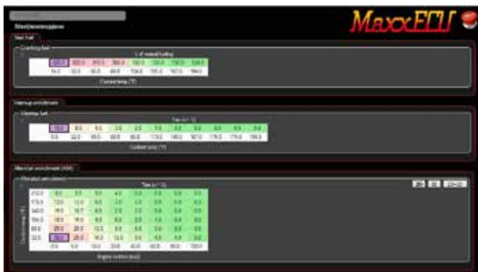
A sample of the tuning parameter tables. This is the ignition advance map that sets the ignition based on the vacuum (an indication of the throttle opening) and engine RPM. Note that at wide open throttle, the ignition advance is reduced from the maximum.
