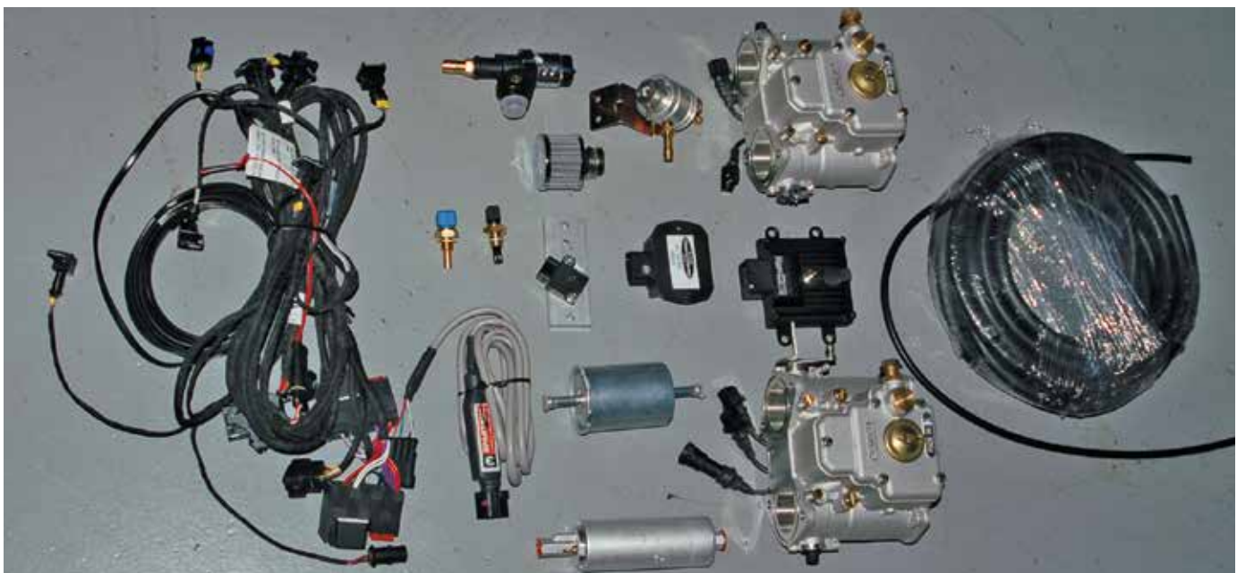
All of the engine management system laid out on the floor
