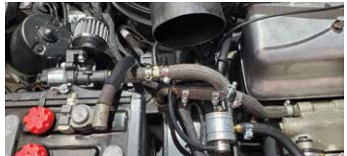
Vacuum (or Manifold Absolute Pressure, MAP) is an important parameter used by the ECU (under the air cleaner), fuel pressure regulator (lower center) and idle air step valve (at left with the small air cleaner).
