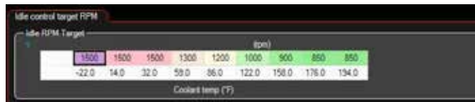
The engine idle speed can be adjusted to varying speeds as the engine temperature rises.
