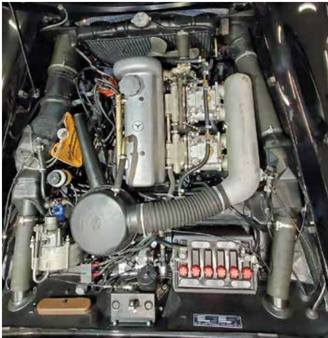
An overall view of the final installation. The Jenvey throttle bodies look very much like Weber DCOE carburetor. Note the fuel rail connects the two throttle bodies and then head to the fuel pressure regulator under the intake hose.
