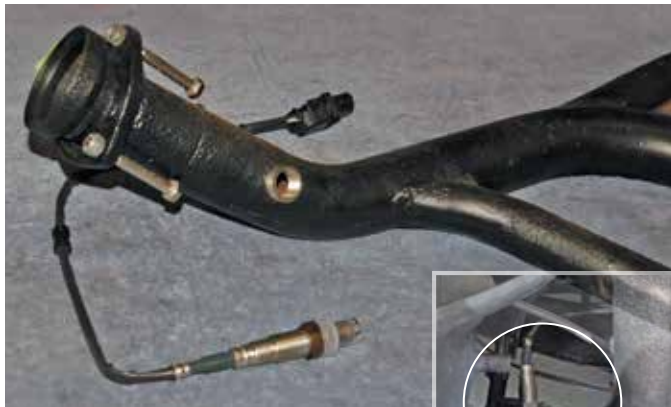
The wide-band exhaust gas analyzer and the exhaust manifold with the analyzer bung located about 20 inches from the exhaust port.
