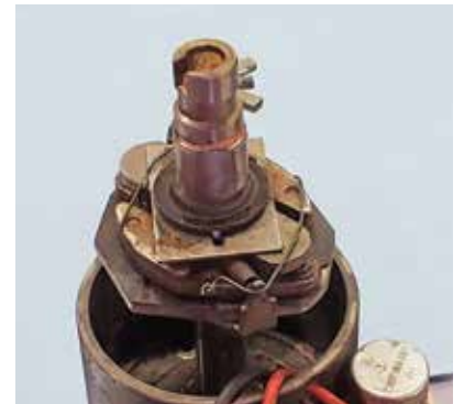
The distributor centripetal advance weights wired in place to inactivate the mechanical distributor advance. The ignition trigger is static at 10 degrees before top dead center.
