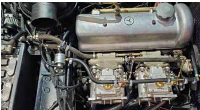
The fuel line connects the two Jenvey throttle bodies and then connects to the fuel pressure regulator. Note that the original accelerator linkage is utilized.
