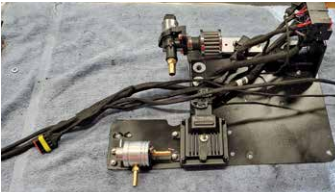
All of the components mounted on the foundation plate. Note that the fuse and relay component is mounted above the idle speed controller.
