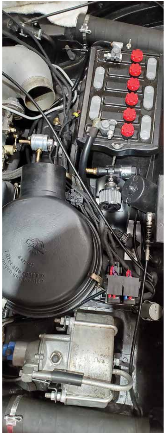
A view of the components with the air filter installed. The idle air step valve with a small air filter is next to the battery and connected to the vacuum pipe.
