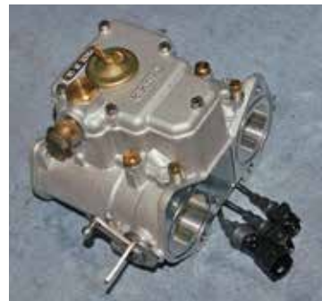
The Jenvey throttle body. It contains two 350cc fuel injectors and a throttle position sensor.
